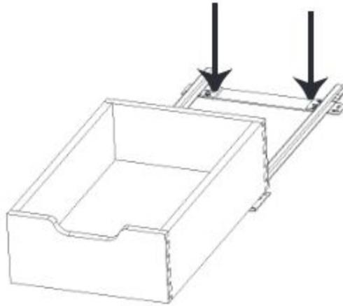
**Step 2.** Slide drawer out half way to allow for installation of rear screws into cabinet floor.
