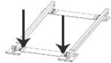
**Step 3.** Slide drawer out completely and lift drawer out of slide structure.
