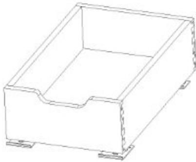
**Step 1.** Place entire unit into cabinet at desired location. Make sure adequate space is available for door closing, etc.
