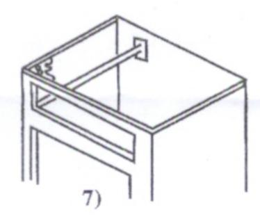
STEP 5: Stand the cabinet upright at this time and attach the 4 plastic Corner Braces in each corner of the cabinet using the &medium screws. The 4 Largest screws are for use in installation on the countertop to the base cabinet through the 4 Corner Braces.
