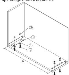
**2.** Mount the side frames to the bottom brackets. Attach pull rod to side frames. Proceed to Step 3.
