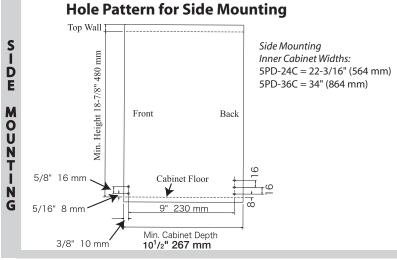
1. Mount the side frames to the walls of the cabinet. Attach pull rod to side frames. Proceed to Step 3.
