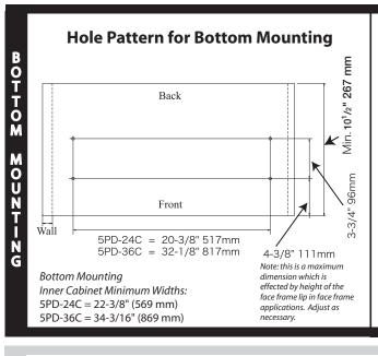
**1.** Mount the bottom mount brackets to the cabinet floor ensuring that bolts with washers are coming up through bottom of cabinet.
